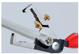
Induction hardened shear blade with precisely ground cutting edges for crushing-free cutting of copper cables up to Ø 15 mm (5 x 2.5 mm²)
